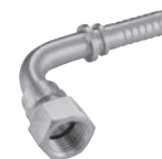
90° Metric Female 24° Cone Seat, L Series with O-Ring DIN 2353
