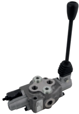
3/8" BSPP, 102 Series, 3 Position, Single Section, Open Centre, 85-175 bar Relief Valve
